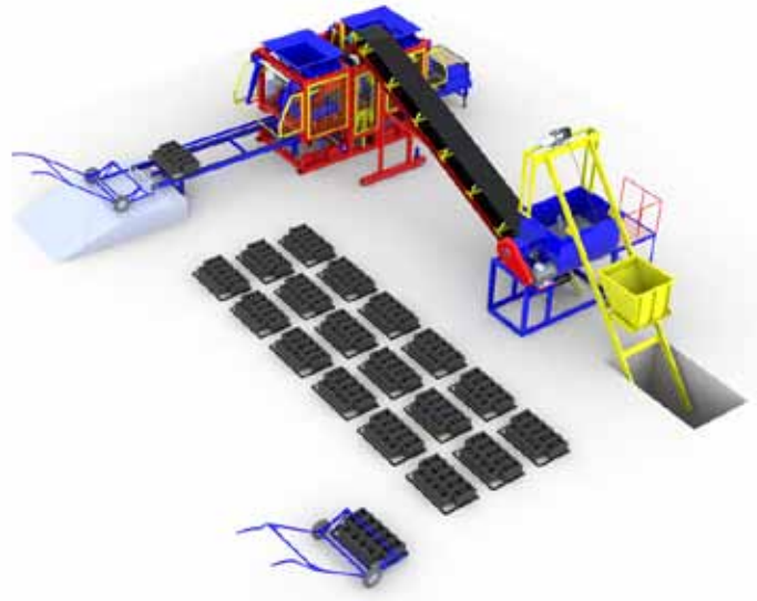
Manuel Beton Parke ve Blok Üretim Tesisi Manual Concrete Pavers and Block Production Facility
