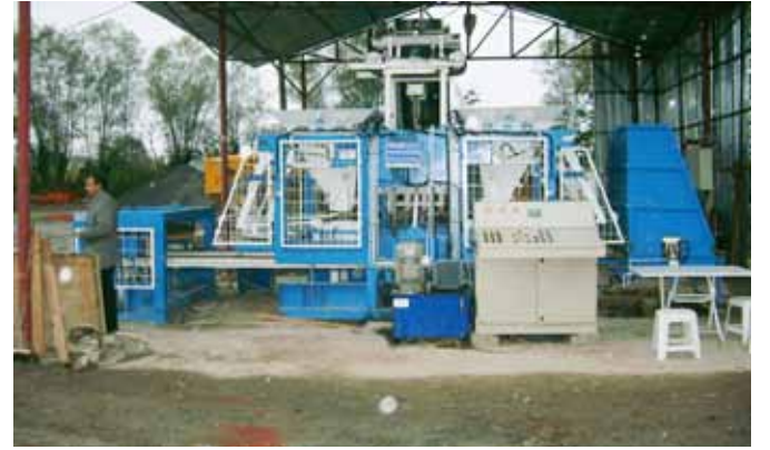
Türkiye - ZIM1025 Beton Parke ve Blok Üretim Tesisi Turkey - ZIM1025 Concrete Pavers and Block Production Facility
