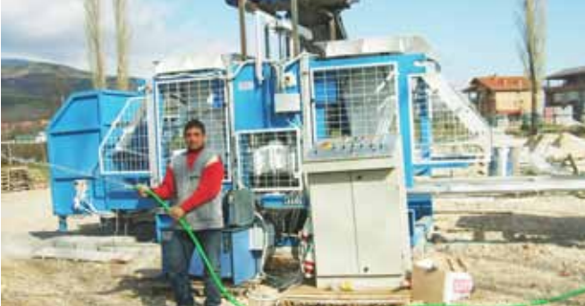
Makedonya - ZIM1025 Beton Parke ve Blok Üretim Tesisi Macedonia - ZIM1025 Concrete Pavers and Block Production Facility
