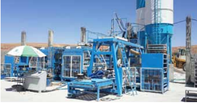
Cezayir - ZIM1025 Beton Parke ve Blok Üretim Tesisi Algeria - ZIM1025 Concrete Pavers and Block Production Facility
