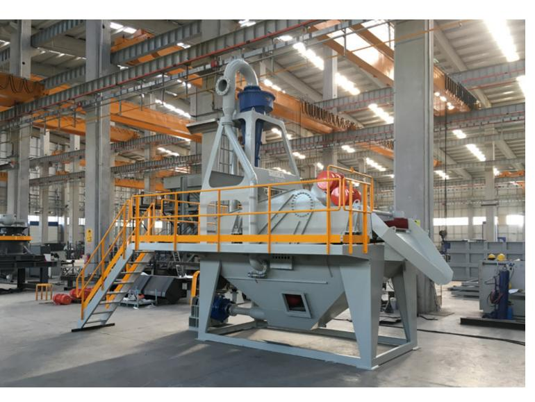
In general applications, an MEKA Sand Unit produces a 0-5 mm (0-4 mesh) washed sand in accordance with applicable concrete sand standards.
