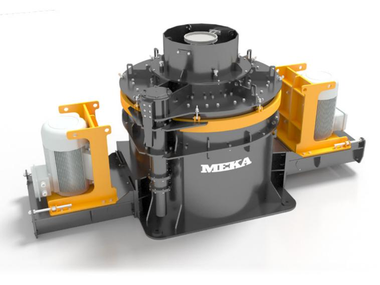
Vertical Shaft Impact (VSI) crushers are designed to be used in secondary, tertiary or quarternary stage crushing. The crushers are suitable for a wide range of applications including the production of high quality manufactured sand, well formed aggregates and industrial minerals. Crushers can also be used for shaping or removal of soft stone from aggregate.
